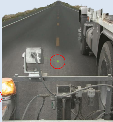
Gun Carriage Guidance - The laser is used to give the operator "heads up" time to move the gun carriage in and out for easy and precise alignment.
